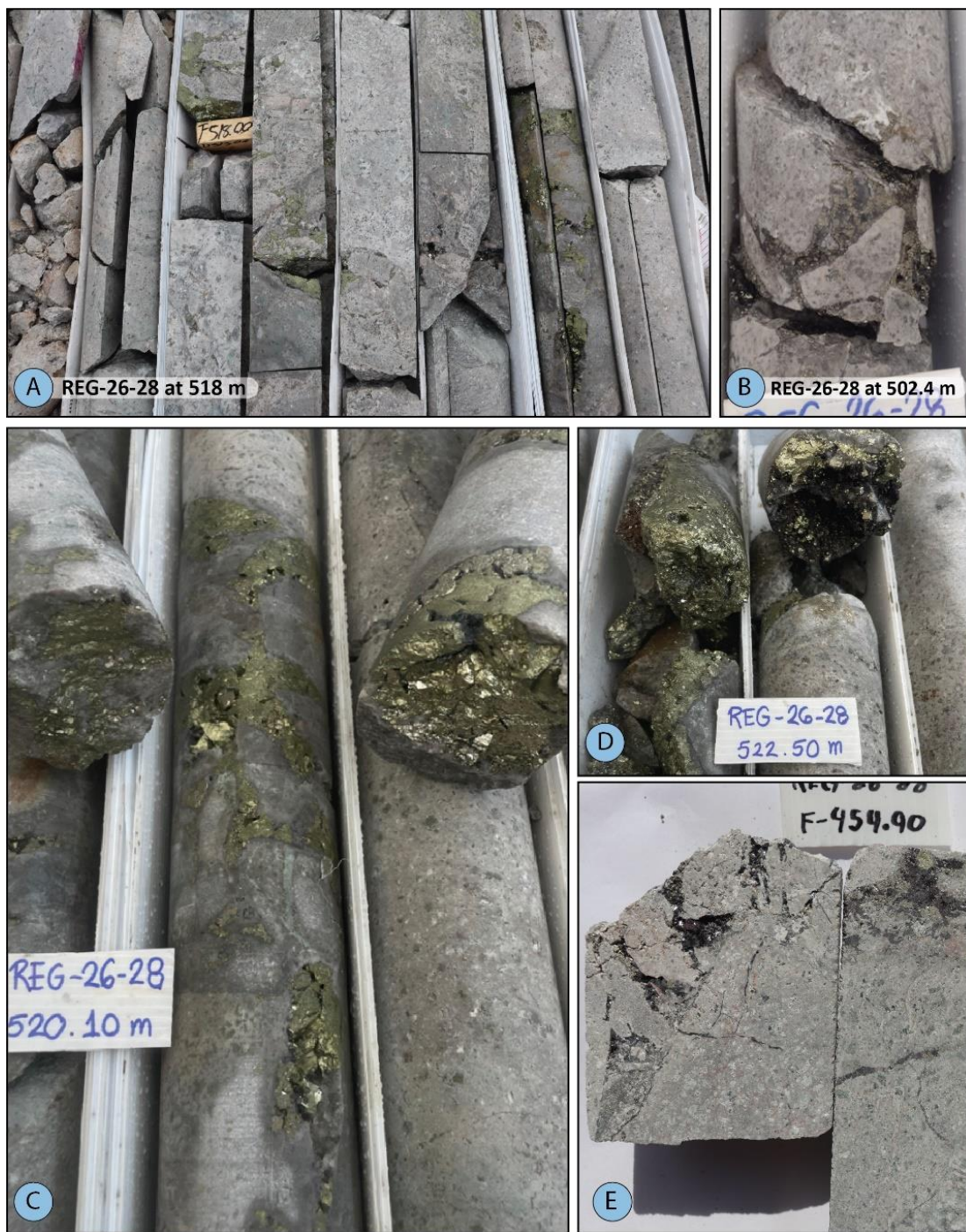
Figure 1: Selection of photographs of the sulphide-specularite infilled breccias from REG-26-28.
