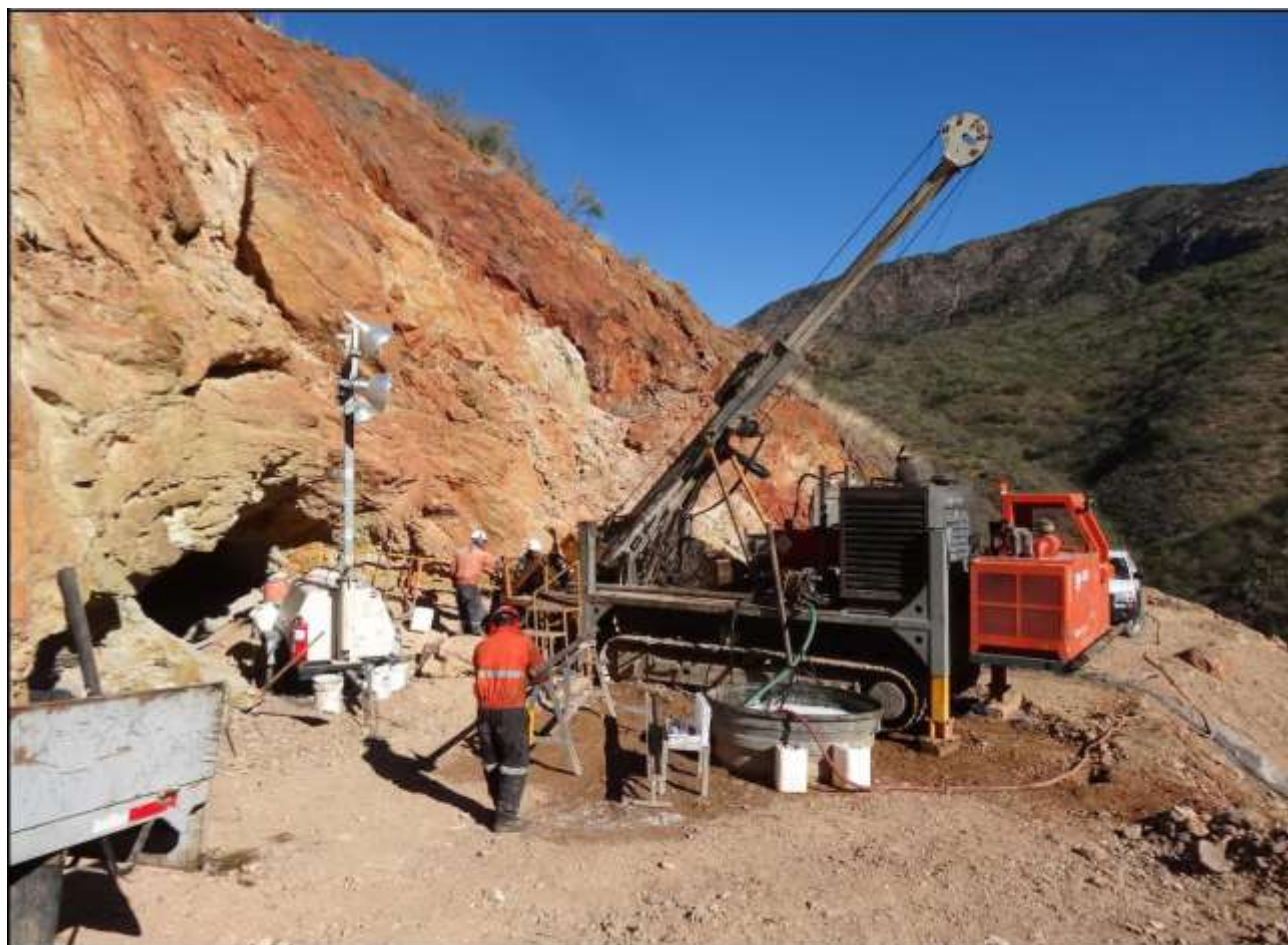
Figure 10-1. Regency diamond drill hole RDP-18-07.
