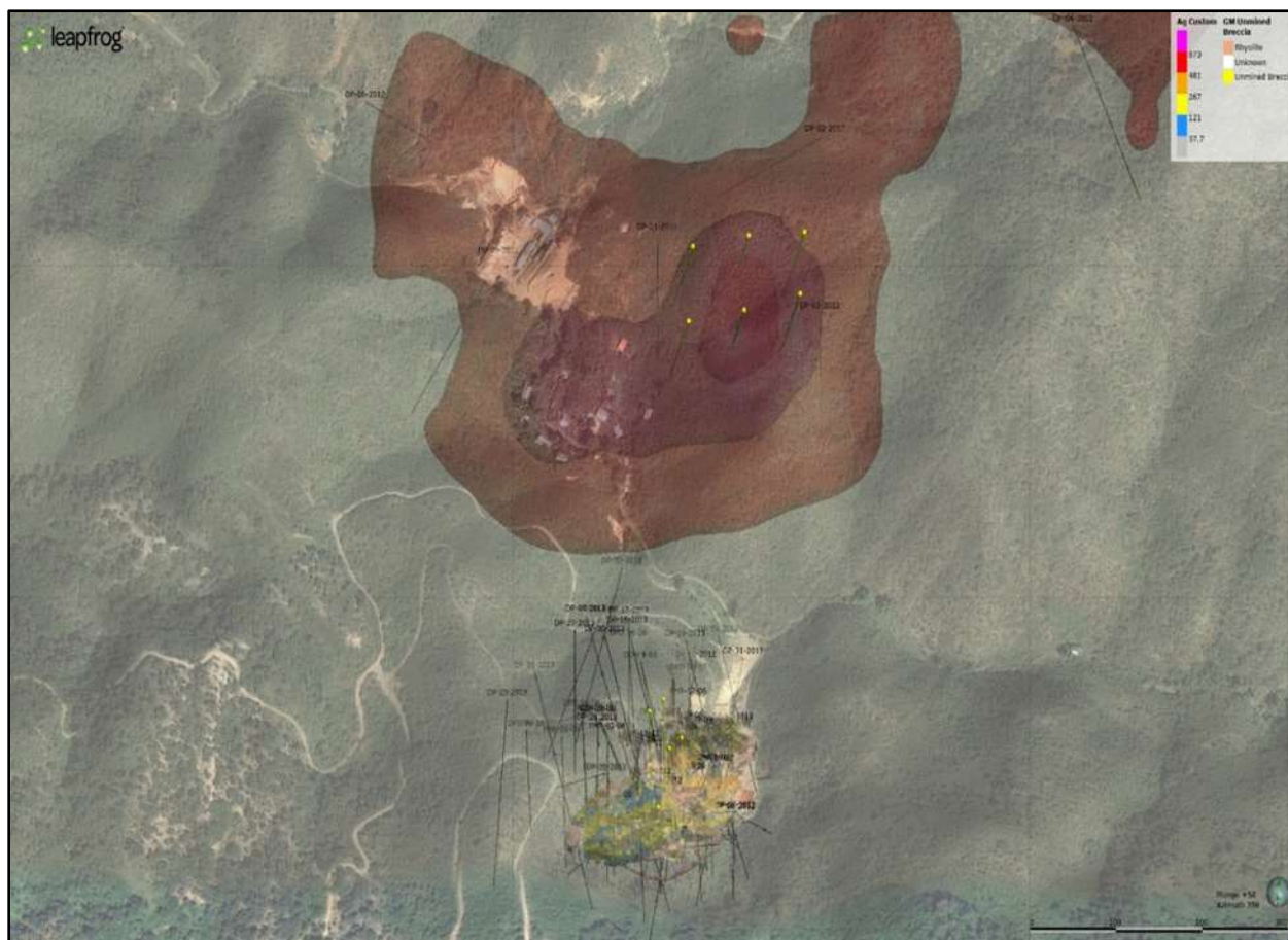
Figure 6.7. Chargeability at 200m below topography. Higher amplitude anomalies are purple shades.
